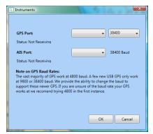
When loading Chart Plotter it looks for the previous connection to the GPS/AIS, this prevents having to reset your data connection every
