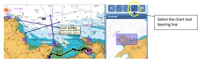
Lines can be drawn on the chart to determine bearings and distances. As the line is drawn the distance and bearing
