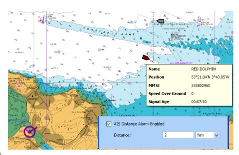
that distance to your GPS position a warning will appear on the screen, also when selecting the AIS tab to list all the AIS messages, the ships within the alarm area are highlighted.
